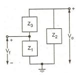
But as the phase shift of the feedback network is  $180^{0}$ ,  $\beta = -\left[\frac{Z_{1}}{Z_{1} + Z_{3}}\right]$
