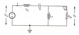
$$V_0 = h_{fe} I_b X_{L2} = h_{fe} I_b j\omega L_2$$
