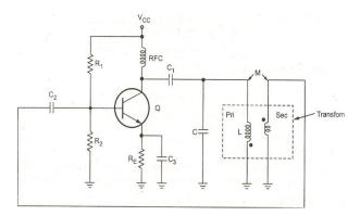
There is mutual inductance M between primary and secondary of the transformer which introduces a phase shift of  $180^0$ , as indicated by the dots, in addition to the phase shift of  $180^0$  by transistor Q. Thus overall phase shift around the loop is  $360^0$  which satisfies the Barkhausen criterion.
