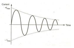
To make oscillations sustain, an amplifier can be used to compensate the energy which is lost.
