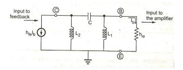
The output current is current  $I_C = h_{fe} I_b$ collector where  $I_b$  is the base current, h<sub>ie</sub> the input impedance of the transistor. The output of the feedback is  $I_b$ , which is the input current of the transistor.
