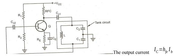
acts as the input to the feedback network. While the base current  $I_b$  acts as the output current of the tank circuit, flowing through the input impedance  $h_{ie}$  of the amplifier, hence the equivalent circuit.
