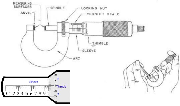
> The part must be held in left hand and the micrometer in right hand.
