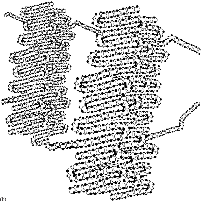
Figure 2.22 (a) Spherulite structure showing the molecular-level lamellar chain-folded platelets and tie and frayed chain arrangements. (b) A more complete description of two sets of three lamellar chain-folded platelets formed from polyethylene. Each platelet contains about 850 ethylene units as pictured here.
